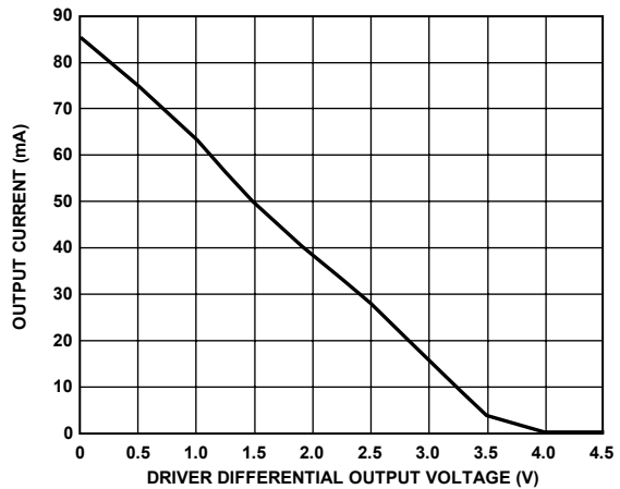
Figure 7. Output Current vs. Driver Differential Output Voltage
